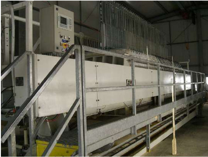
Figure 6: Sand processing Mill, near Provodin, Czech Republic. Water is used to wash mined sand, then is drained into tanks, filtered, and recycled.
